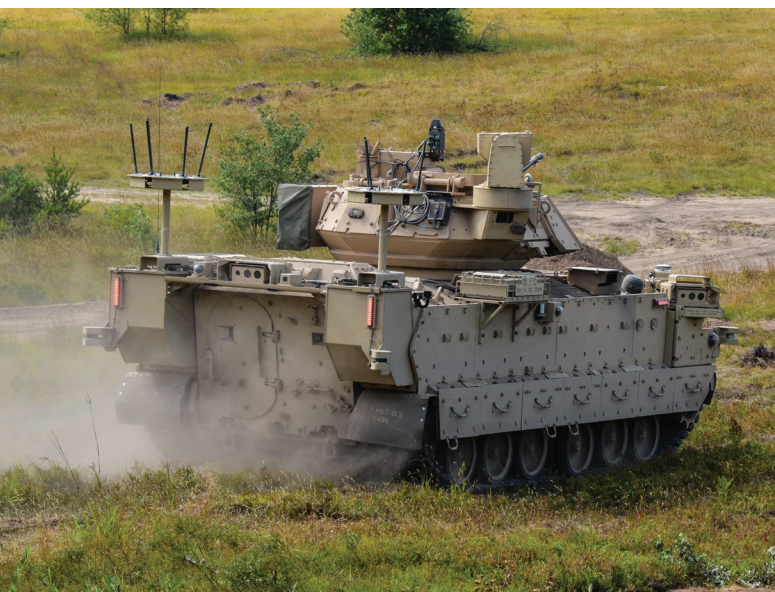
The Mission Enabling Technologies Demonstrator manned vehicle can control two unmanned platforms. (Photo Credit: U.S. Army)
